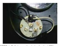
STEP 4: Drill 4 mounting holes for the LED's, using a 5/32" drill bit, at desired locations. Insert LED's in hole from front of panel.
