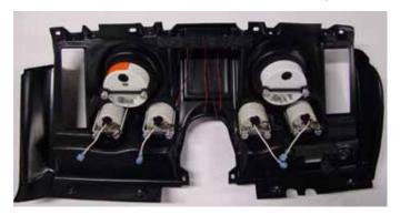
STEP 2: Install appropriate lamp socket pigtails into the gauges. Follow specific instructions for the tachometer and speedometer as the are several different lighting configurations.
