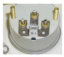
STEP 1: Install the blade terminals to the back of each of the 4 small gauges. Secure with lock washer and nut. There are specific left, center, and right hand terminals. Install as shown in photo.
