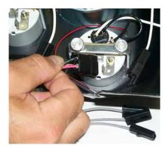
STEP 5: Plug in gauge connections using supplied connectors. Plug in connectors in the order shown below.
